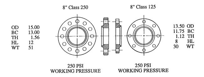
Note: Class 250 flanges have raised faces. If Class 250 flanges have raised faces, they should not be mated with flat faced Class 250 flanges.
