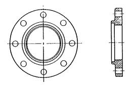
These flanges are adequate for water service of 250 psi working pressure. Bolt circle and bolt holes can be joined with Class 125 ANSI B16.1 or Class 150 ANSI B16.5 flanges. However, these flanges cannot be joined with Class 250 ANSI B16.1 flanges, flanged fittings and valves.
