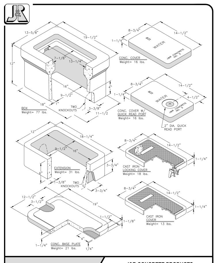
No. W3 Series Meter Box Designed for 5/8" or 3/4" Meters
